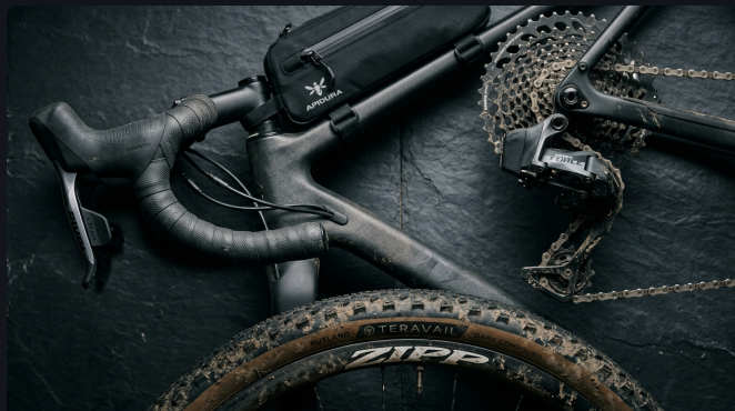
SRAM Force AXS wireless transmission with massive 10-52T cassette and Teravail 47mm casing.
